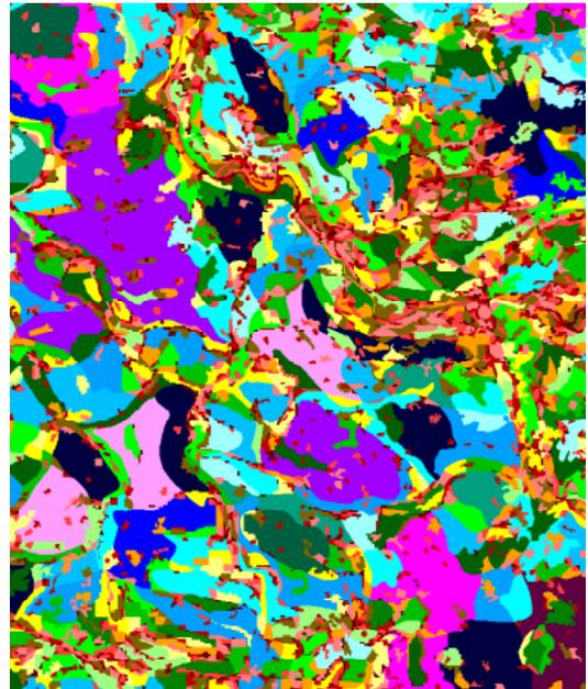
**Fig. 2:** Section of about 85 x 70 km of the elementary units (EU) map generated for the German part of the Elbe basin. The total map consists of 64.550 EUs.
